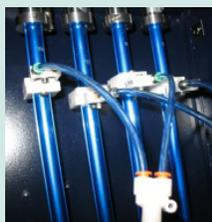
Incisive Surgical relies on the CVT-P-10 pneumatic vibrator to assist the material flow of INSORB Staples from a molding machine through a 35" tubes where they are stored, and later moved to another location.
